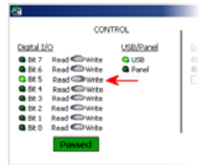
Figure 11-7: Bit 5 - Normal Logic Input
