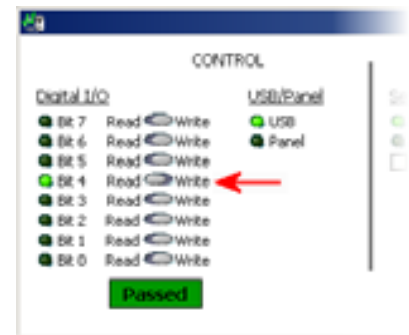
Figure 11-6: Bit 4 forced Low
