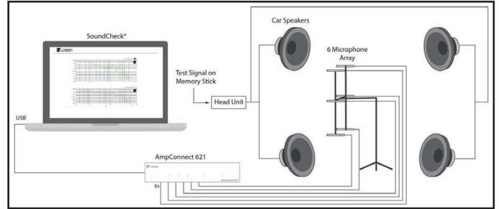
Figure 1: Test configuration for measurement of Max SPL and Max SPL Spectrum
