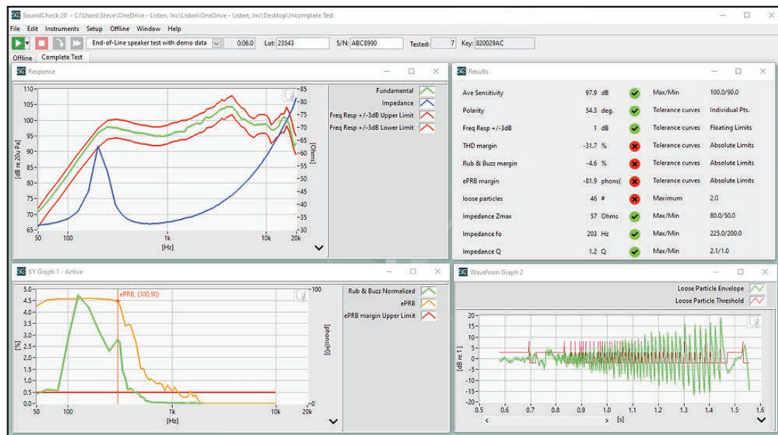
Figure 2: Typical end-of-line tests for a loudspeaker showing frequency response, sensitivity, polarity, THD, Perceptual Rub & Buzz, loose particles, impedance, and resonance
