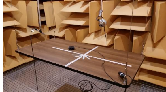
Figure 5. IEEE 1329-2010 test setup used (full anechoic chamber)
