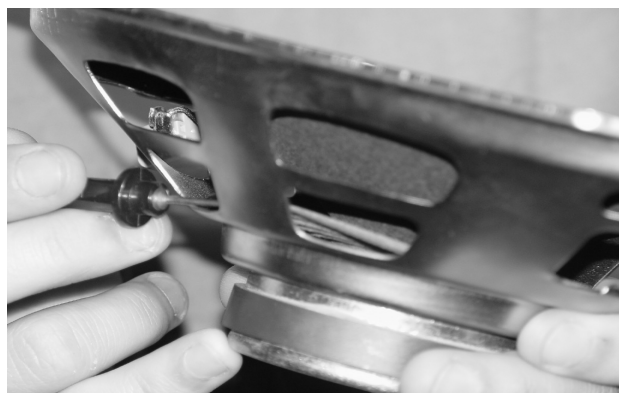
Figure 8: Spider improperly glued
