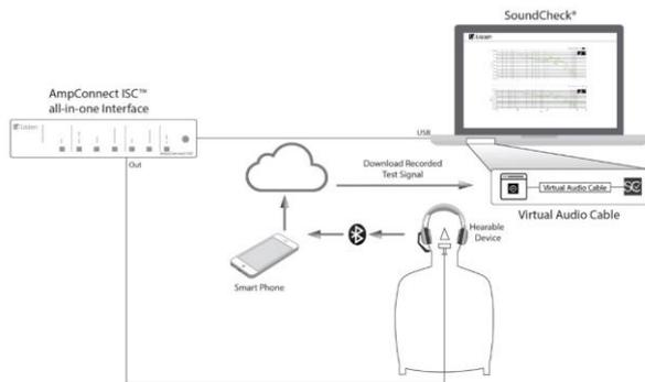
Figure 8. Test configuration for headset microphone measurement using voice activation
