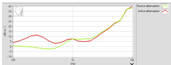
Figure 11. Typical Noise Cancelling Measurement Results
