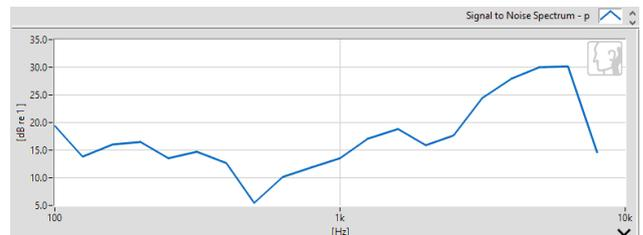
Figure 14. SNR for a smart headset measured with ETSI standard background noises
