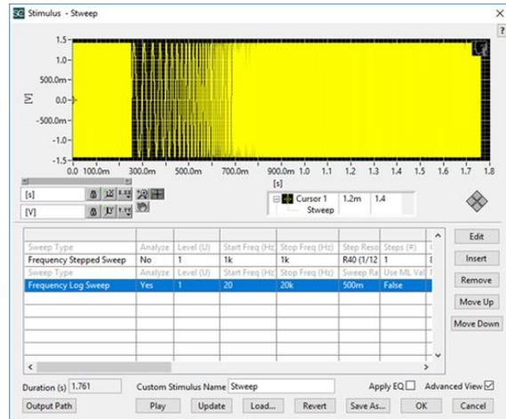
Figure 7: 1 kHz frequency tone prepended to stepped sine stimulus to calculate sampling rate and simplify record triggering
