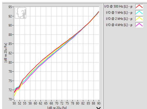
Figure 16. Hearable measurement of Input vs. Output
