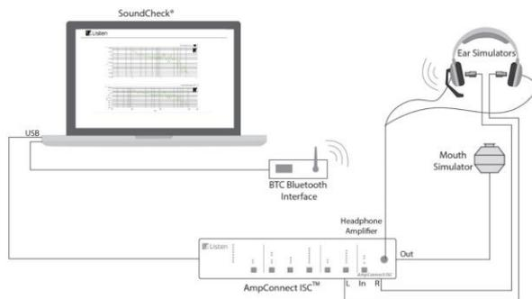
Figure 1. Test configuration for basic wired and wireless (Bluetooth) headset measurement
