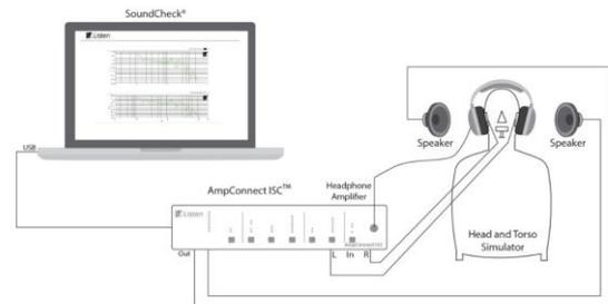
Figure 10. Test configuration for measuring ANC headphones
