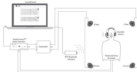
Figure 13. Test configuration for headset measurements with ETSI standard background noises
