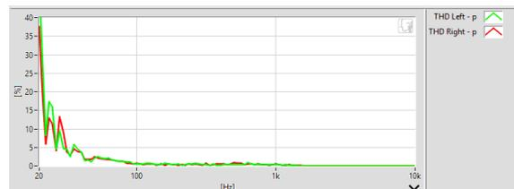
Figure 4. Smart headphone distortion response
