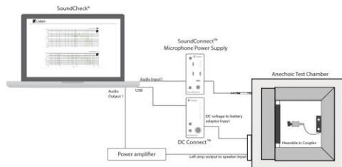
Figure 15. Test configuration for measuring hearing aids
