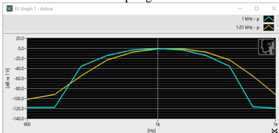
Figure 6. Recorded waveform needs to be resampled to match sample rate of test signal
