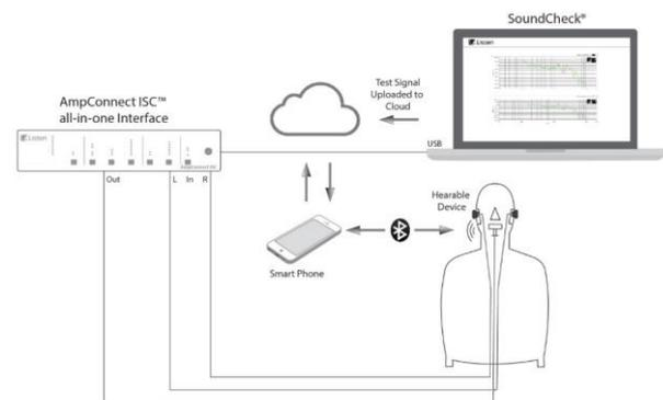
Figure 2. Test configuration for stereo headphone measurement using voice activation
