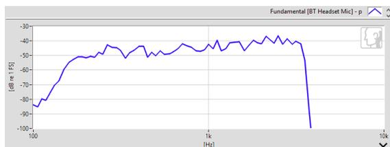
Figure 9. Frequency responses of hearable microphone array
