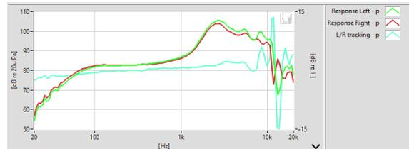
Figure 3. Smart headphone frequency and left/right tracking responses
