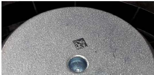
Figure 18. Sample inkjet printed datamatrix code
