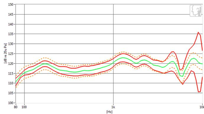
Figure 17. Engineering  $\pm 3$ dB frequency response specification (dashed orange) and typical EOL manufacturing  $\pm 5$  sigma limit (red)
