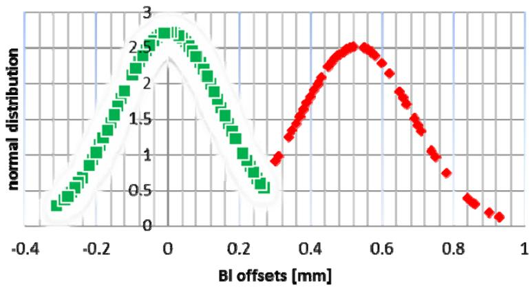
Figure 6. Two batches of speakers produced with different spider to VC settings
