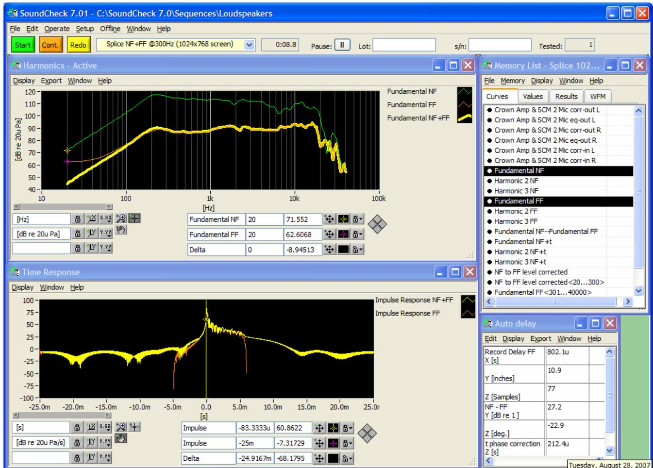
**Top graph: Near Field, Far Field, and Spliced Frequency Responses, Bottom graph: Time-windowed Far Field and Spliced Impulse Responses Table: Mic distance, NF and FF level and phase difference**
