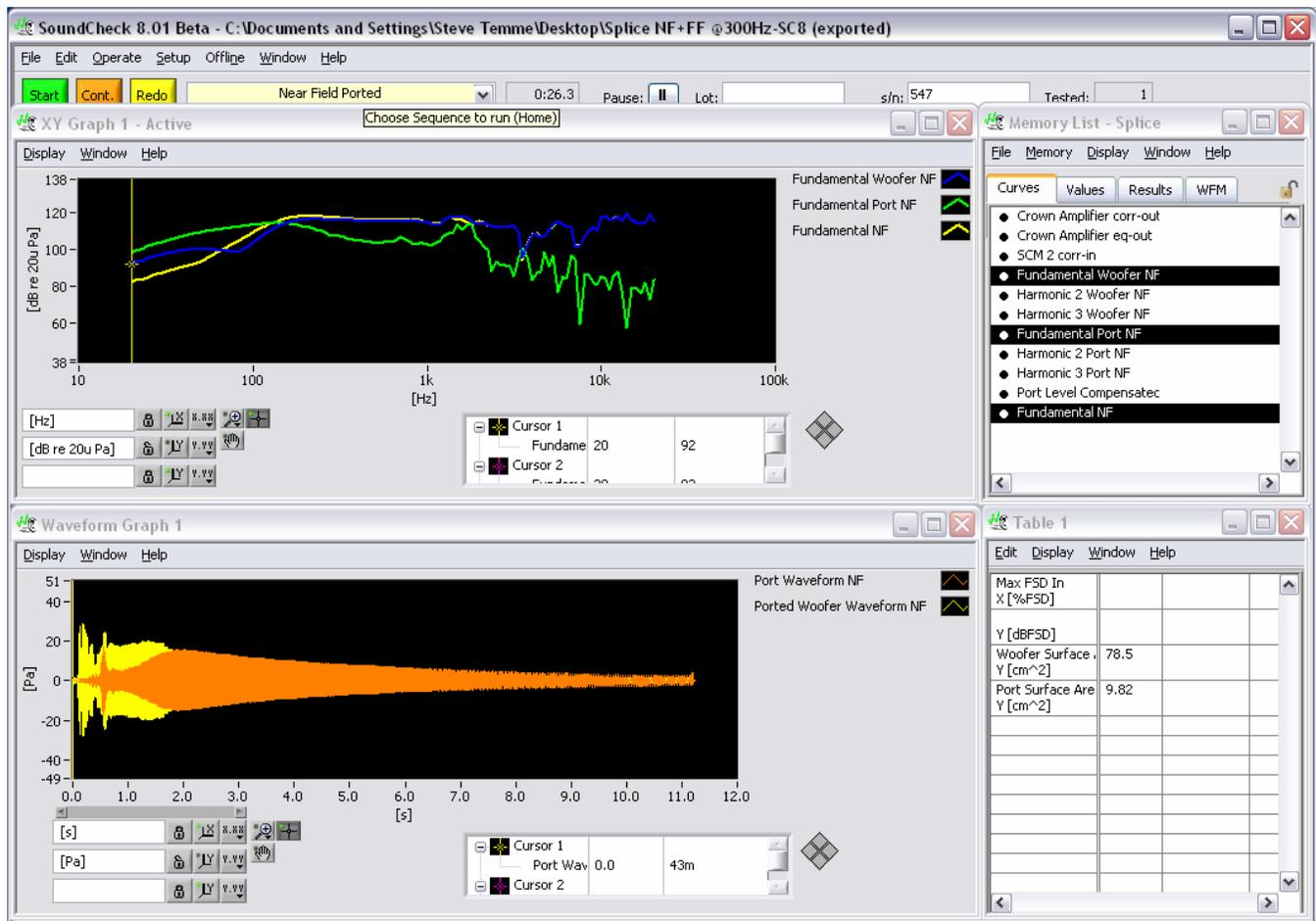
**Top graph: Near Field Response of both Woofer and Port, Bottom graph: Recorded Time Waveforms of both Woofer and Port, Table: Calculated Woofer and Port(s) surface areas**
